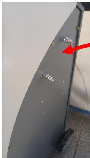
RETIRE A TAMPA LATERAL DA TD 7020 PARA TER ACESSO AO FILTRO SECADOR.
